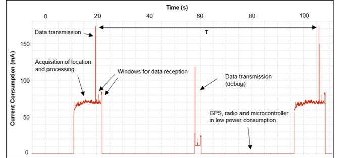
Fig. 8. Device current consumption profile in Data Transmission Mode. There is a transmission for control and debugging between data transmissions that can be ignored.
