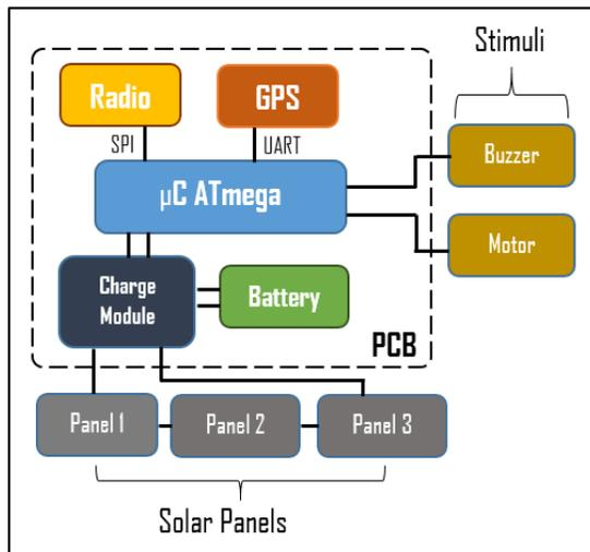
Fig. 2. Block diagram of Sensor Node (SN).
