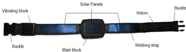
Fig. 7. Final prototype of SN.
