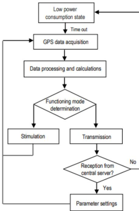
Fig. 3. Simplified flowchart of the SN embedded software.
