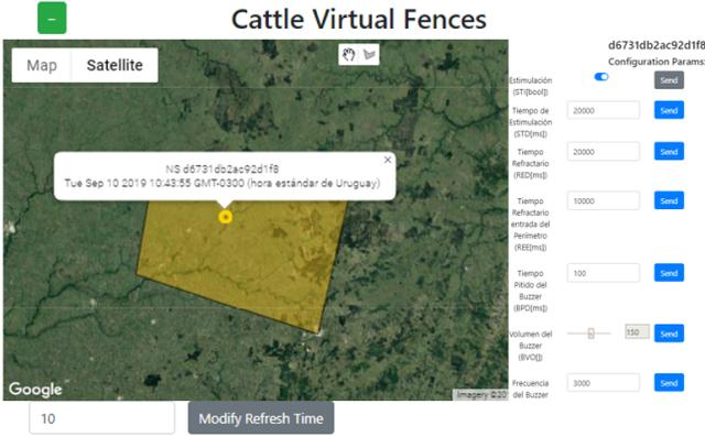
Fig. 6. SN location and virtual fence configured in the user interface.
