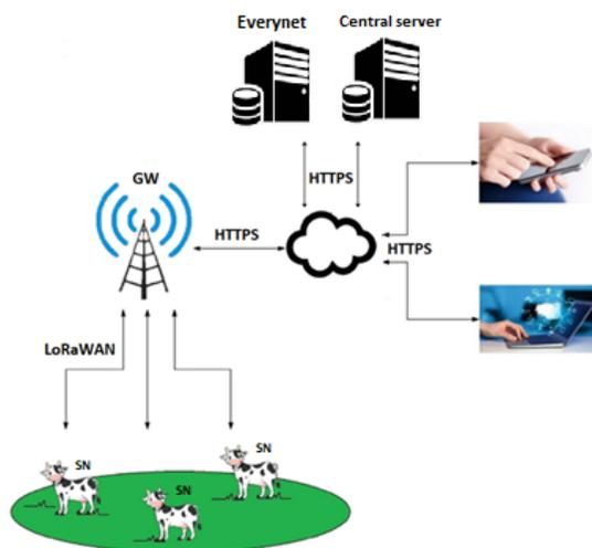
Fig. 1. Architecture of the proposed solution.
