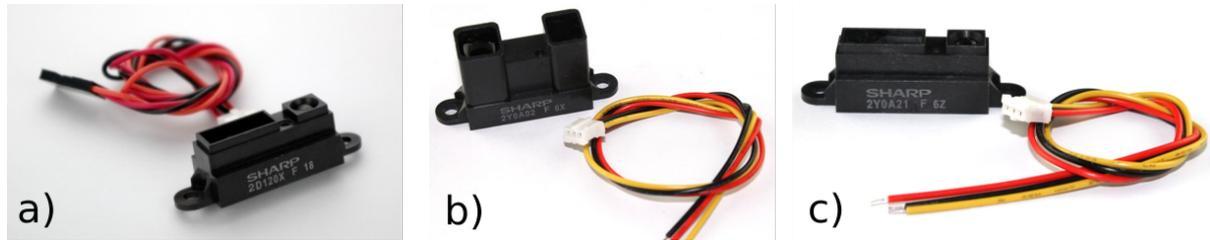
Figura 3.12: a) Sensor Sharp-gp2D120X. b) Sensor Sharp-2Y0A02. c) Sensor Sharp-2Y0A21.[43, 44, 45]
