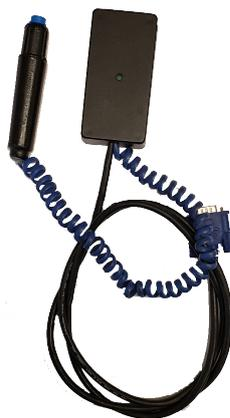
Figura 7.5: Consola de test.
