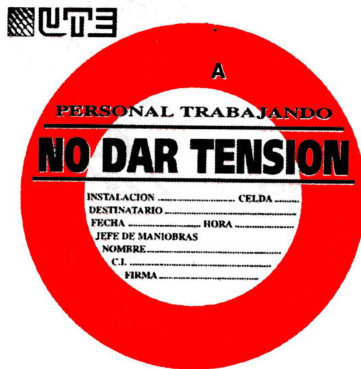
Figura 8.2: Cartel Disco "NO DAR TENSION"
