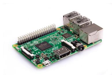
Figura 5.1: Raspberry Pi Modelo 3 B [63]
