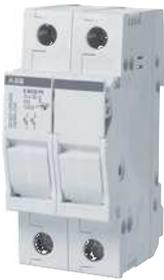
E 90 PV series fuse disconnectors (UL approved), designed for operating voltages of 1000 V d.c. with utilization category DC-20B, are particularly suited for protection against overcurrents of photovoltaic systems. The single-pole or two-pole E 90 PV disconnectors for 10.3 x 38 mm cylindrical fuse links offer a reliable, compact and affordable solution for photovoltaic installations. Versions with blown fuse indicator allow to check whether the fuse is still working correctly or not.
