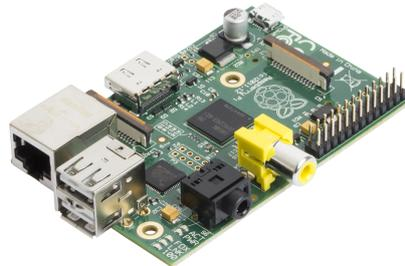
Figura 7.1: RaspBerry Pi Model B.
